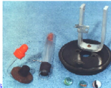
Parts of the test-tube engine.
