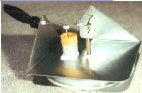
One-moving-part, test-tube Stirling engine. Parts of the test-tube engine.
